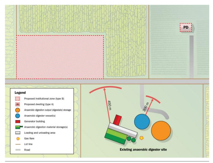
Figure 5. Implementation Guideline #22 — MDS I setbacks for anaerobic digesters.
