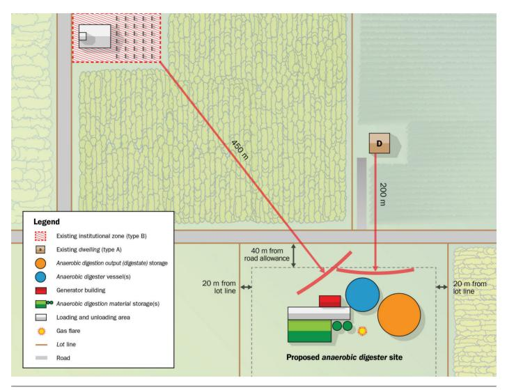
Figure 6. Implementation Guideline #22 — MDS II setbacks for anaerobic digesters.
